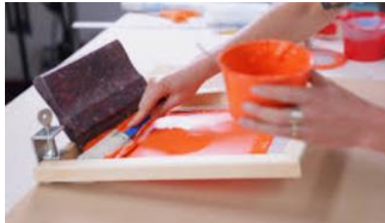
Step 3. Place the ink on one edge of the stencil.
